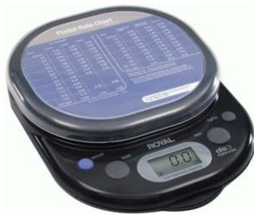
Figure 4. The simple postal scale used to monitor the applied force of the stimulator.
