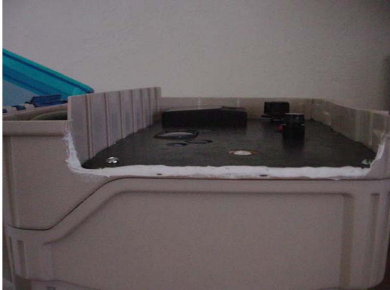
Figure 8. Side view showing level mounting of vibrating stimulator.
